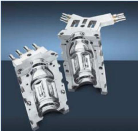
Patented quick change technologies for hotfill application.
